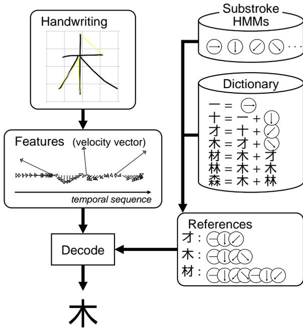
Figure 1. System configuration.
