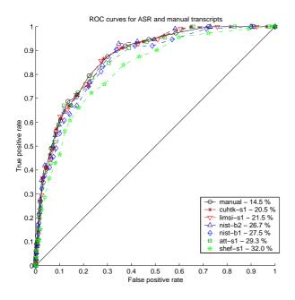
**Fig. 3.** The influence of various WERs on the speech data summarisers - ROC curves for summarisers corresponding to different quality ASR transcripts plus the manually-generated transcript. WERs for the ASR and manual transcript are measured against 10 hours of TREC-8 reference data [15].
