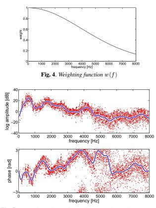
**Fig. 5**. Spectral envelopes of one of the articulatory clusters computed using the piecewise constant approximation
