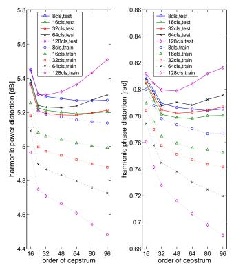
Fig. 7. Harmonic distortion vs. order of cepstrum, in the case of the piecewise linear mapping
