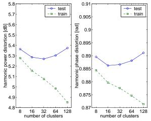
Fig. 3. Harmonic distortion vs. number of clusters, based on cepstral domain criteria for the piecewise linear mapping
