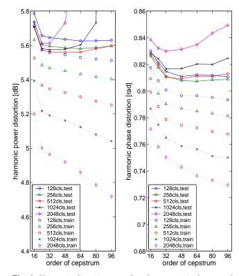
Fig. 6. Harmonic distortion vs. order of cepstrum, in the case of the piecewise constant mapping
