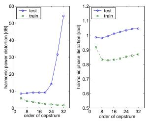
Fig. 1. Harmonic distortion vs. order of cepstrum, when each cluster comprises only one frame
