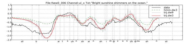
Fig. 2. Recovered trajectory for the movement of Upper Lip in x coordinate (ul\_x) of test utterance fsew0\_006. The trained trajectory HMM (trj.dw3) shows a closer fit to the data than the baseline HMM (trm.dw3), with state alignment derived from a 8-mixture jointly trained 2-stream HMM. The light gray trajectory of (trj.dw9) shows the noisy effect of using 9-frame dynamic window.
