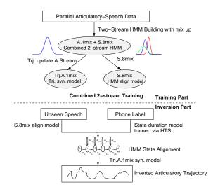
Fig. 1. Overview of the articulatory-acoustic modelling system. Using twostream combined training results in greater accuracy compared with the separately trained ones.
