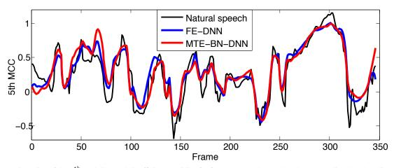
Figure 1: Trajectories of the 5<sup>th</sup> Mel-Cepstral Coefficient (MCC) of reference natural speech and those predicted by baseline FE-DNN and proposed MTE-BN-DNN systems.
